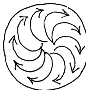
Hot gases spiral up a flue. A round flue will carry more gas, more smoothly.
