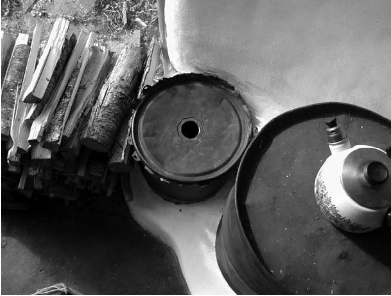
The Rocket Stove in Ianto Evans's cottage, seen from above. Dry firewood, cut thin, the small feed barrel with lid and the large heat riser barrel with tea kettle.
