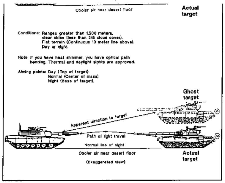
Figure 1-17. Optical path bending in the desert.
