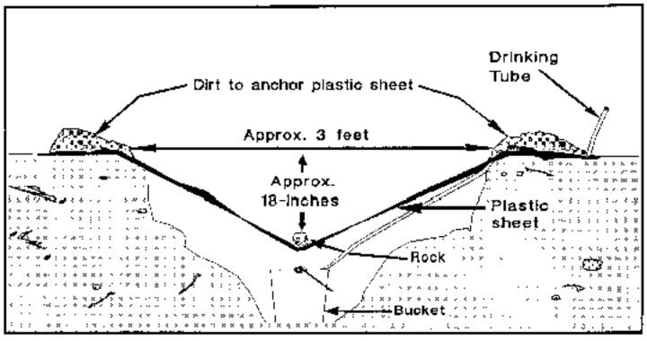
Figure 1-15. Cross-section of a survival still.
