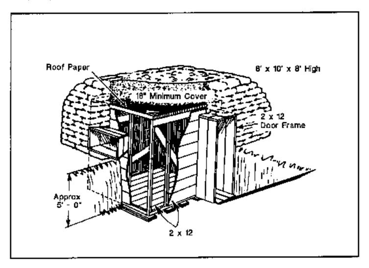
Figure 3-4. Command bunker.
