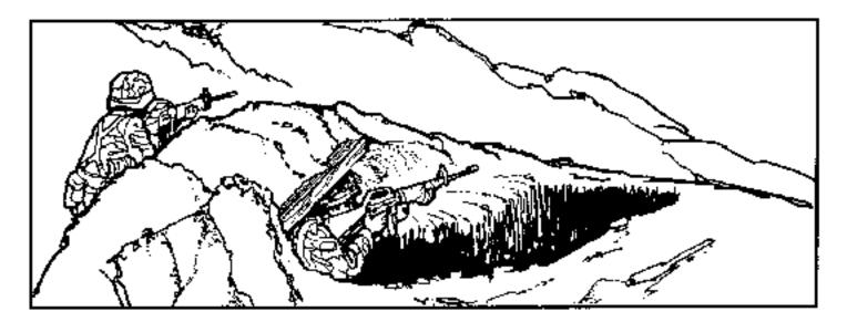
Figure 3-2. Two-man fighting position with overhead cover.
