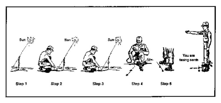
Figure 2-1, Finding direction using shadow-tip method.
