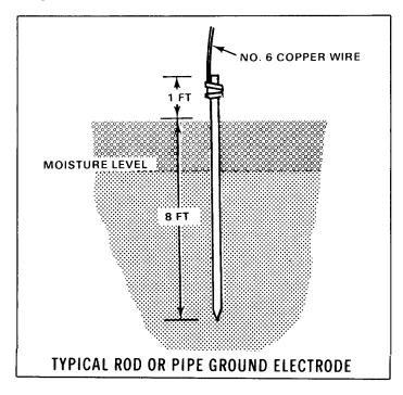
If one grounding rod does not produce a good grounding system, the operator can form a network with three or more rods. Install the rods about 6 feet apart. If three rods form the network, place them in a straight line or in a triangular pattern. Install more than three rods in a straight line. Connect the grounding cable from the generator set to each grounding rod so they are in series.
