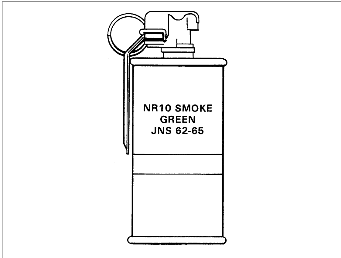
Figure F-5. JNS 62-65 smoke hand grenade.
