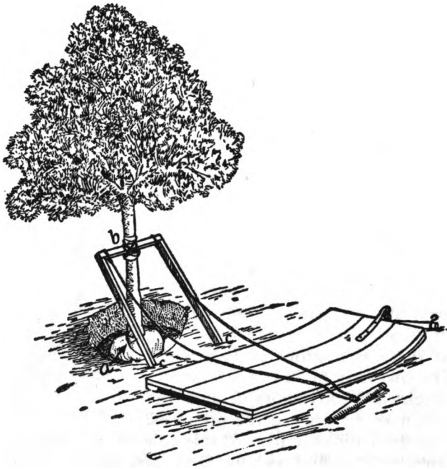
RIG FOR MOVING TREE
