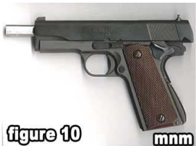
Full cock the hammer and then pull the slide to the rear until the rear of the slide release lever is directly under the rear, small, circular notch in the slide.
