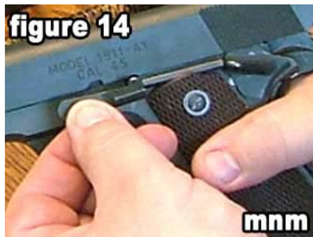
Pull the slide stop towards you, removing it from the slide .
