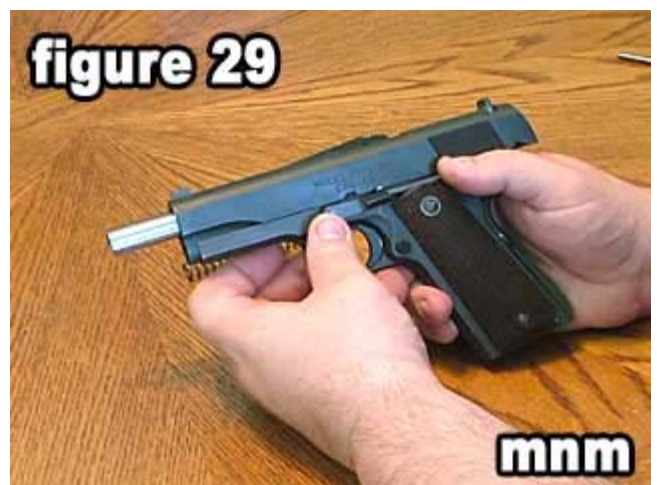
Insert the pin of the slide stop into the slide stop hole.
