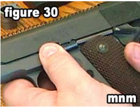
While pressing in the slide stop it may be necessary to slightly compress the plunger so the slide stop snaps into place.
