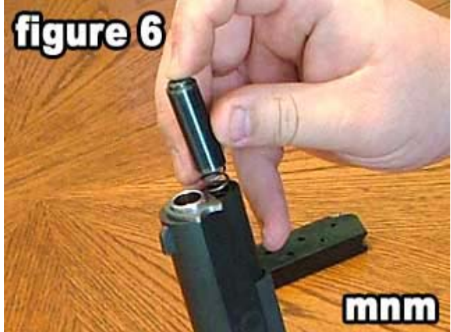
Allow the recoil spring to slowly expand to its fullest extent.
