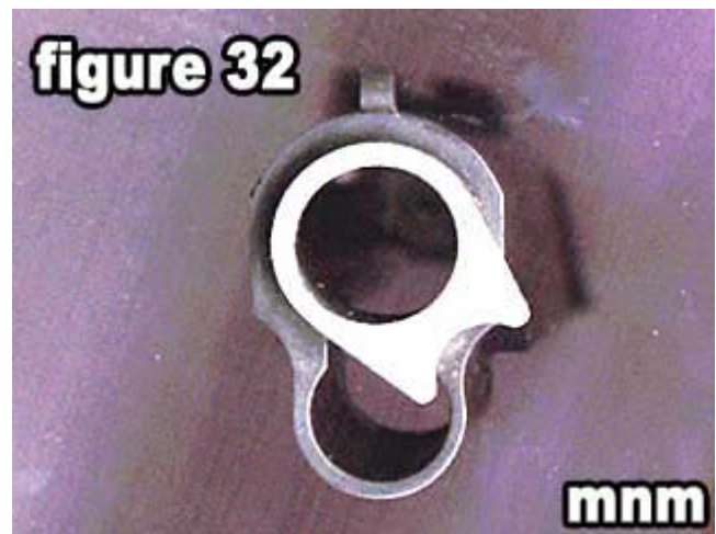
The position the barrel bushing needs to be in to be inserted into the slide.
