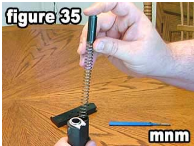
Insert the recoil spring and recoil spring plug.
