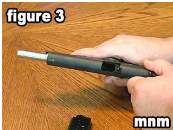
Pull back on the slide and ensure there is not a cartridge loaded in the chamber.
