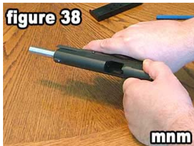
Cycle the slide to ensure proper operation.
