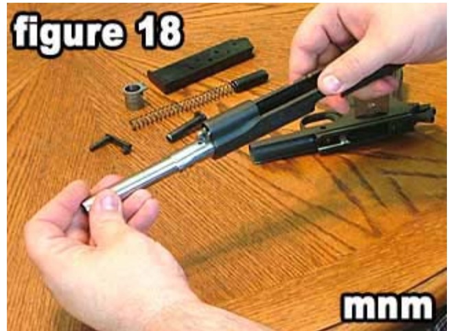
Pull the barrel assembly out of the front of the slide and set aside.
