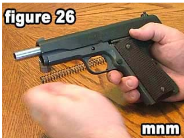
Pull the slide back until the rear, small, circular notch in the slide aligns with the rear slide hole.
