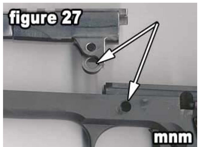
The slide stop hole and the barrel linkage hole.
