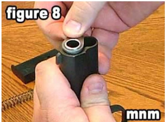
Turn the barrel bushing counter-clockwise.
