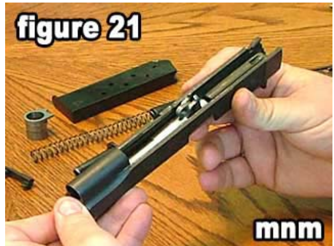
Slide the barrel assembly all the way to the rear.
