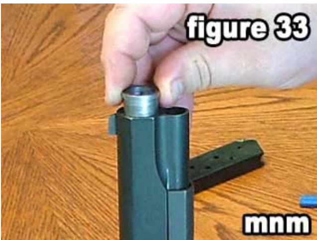
Insert the barrel bushing and rotate clockwise all the way.
