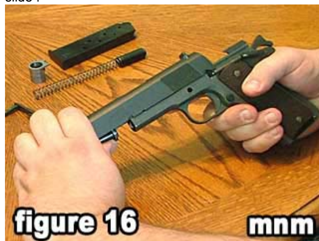
Slide the slide forward and off of the receiver frame.
