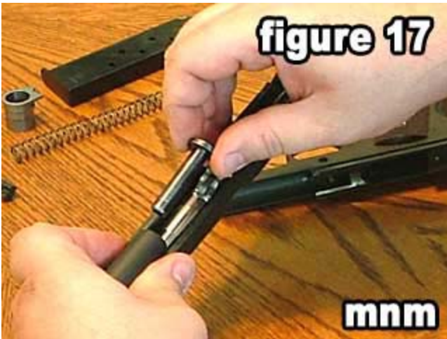
Remove the recoil spring guide and set aside.
