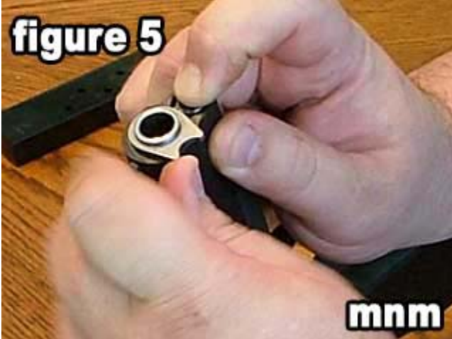
While continuously pressing down on the recoil spring plug, turn the barrel bushing clockwise so the recoil spring and recoil spring plug can exit the slide..
