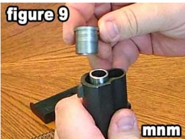
Remove the barrel bushing and set aside.
