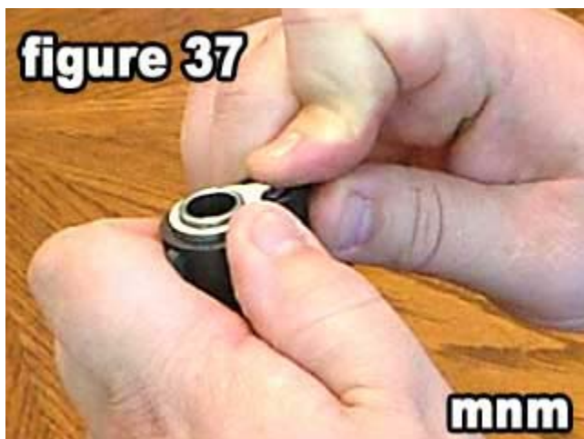
While holding the recoil spring plug down, rotate the barrel bushing counter-clockwise until the barrel bushing locks the recoil spring plug into place.
