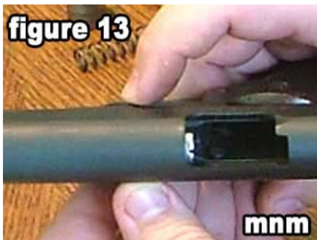
Depress the slide stop pin on the right side of the frame.
