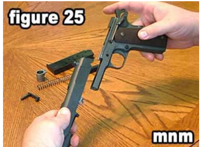
While holding the recoil spring guide in place, place the slide onto the frame's rails.
