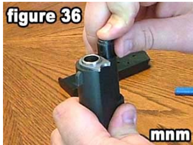
Compress the recoil spring and recoil spring plug.
