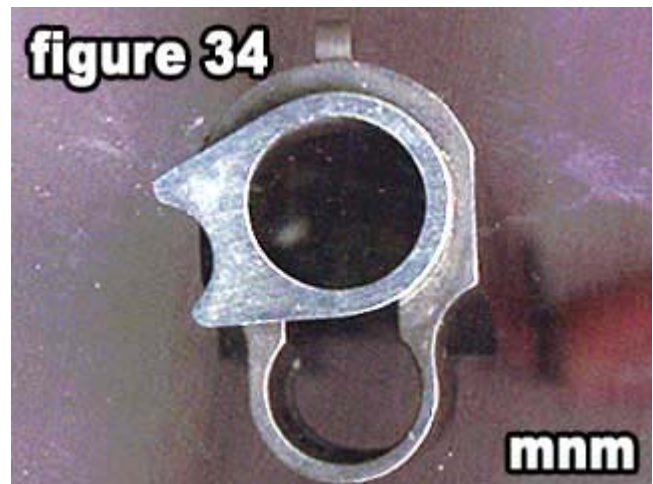
The position the barrel bushing needs to be in for you to be able to insert the recoil spring and recoil spring plug.
