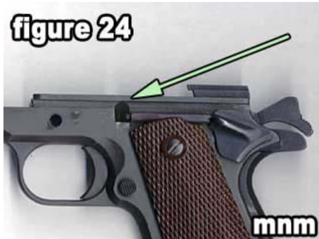
Note the arrow pointing to the rails on the side of the frame. The rails are what the slide rides upon.
