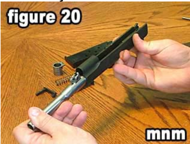
Slide the barrel assembly into the slide as shown.
