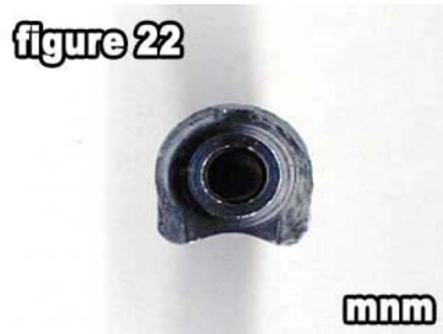
The rear of the recoil spring guide. Note the inward curved bottom. This curved part rests against the barrel.
