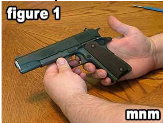
Point the pistol in a safe direction and depress the magazine catch.
