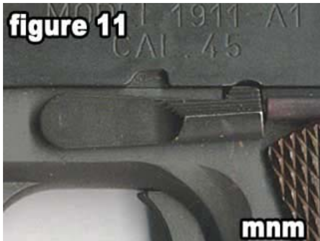
Slide release lever directly under the rear, small, circular notch in the slide.
