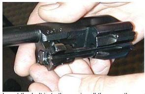
Insert the bolt in to the carrier all the way, then rotate it counterclockwise, while moving it forward along the carrier. Keep it there while inserting the carrier back into the receiver.
