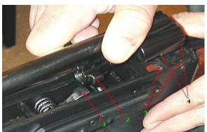
Manually cock the hammer (1) to allow for a carrier to be reinserted. Insert the gas piston end of a carrier into the rear sight block, and lower the rear end of the carrier into the receiver, making sure that the bolt stays in front-locked (2) position inside carrier, and the carrier rear end (4) is aligned with the opening in the receiver railing (3). Push down and forward on the rear end of the carrier to slide it all the way toward the rear sight block.
