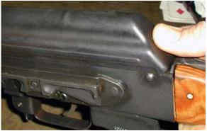
Remove the top cover of the receiver. With your thumb, deep the square serrated button on the end of a top cover, and then lift up the rear end of the cover. Notice, how the front end of the cover was secured in the rear sight block.
