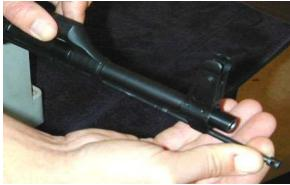
Insert the field tool kit in to the stock, thin end first. To do it real fast, insert it half way, and then slap it with your palm, so that it rides all the way in. Insert the cleaning rod. Make sure that it is locked in it's well.
