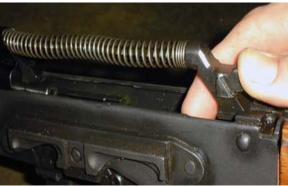
Remove the spring assembly. To do that, once again, push the button on the top end of a receiver to move the spring assembly forward, till it comes out of its well. Notice, how the spring assembly was inserted into the carrier.
