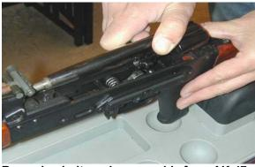
Removing bolt carrier assembly from AK-47 rifle. It has cleared the cuts in the receiver and is being lifted away from receiver. Now you just slide it back, out of the gas tube. Slide the bolt carrier assembly to the rear of the receiver. It will then be aligned with slots cut into the receiver, and you will be able to lift the rear of the carrier upward and remove it by sliding it backwards out of the gas tube (the hole below the rear sight).
