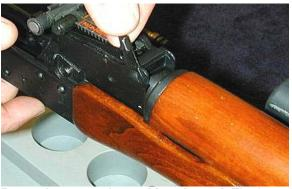
**Removing gas tube and handguard.** The lever has been rotated and the rear of the gas tube raised.
