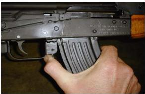
Removing the magazine from the rifle. You press the release with your thumb and rotate the bottom of the magazine forward. Remove the magazine. Then set the safety to "fire" and pull the charging handle all the way back and hold it. While holding the charging handle, visually make sure there is no round left in the chamber If there is no round, release the charging handle and let it slam forward. Pull the trigger.
