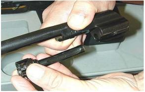
**Removing bolt from carrier.** The tapered lug is now clear of the groove in the carrier, and it is ready to move forward (left in the photo), out of the carrier.
