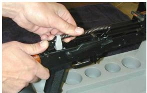
Removing the action (return) spring from AK-47 rifle. It's moved forward and almost disengaged from its grooves in the receiver.
