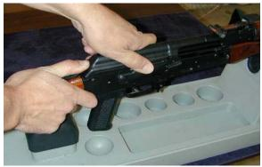
Removing the receiver cover from AK-47 rifle.
