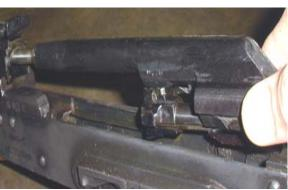
**Remove the bolt carrier.** Safety lever is in "Fire" position, and pull the charging handle all the way back, then lift it up and out of the receiver.
