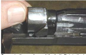
Separate the carrier and the bolt. Rotate the bolt clockwise, and then pull it out of the carrier. Turn the bolt carrier assembly upside-down. Slide the bolt rearward in the carrier. It will rotate and when the tapered bolt lug is aligned with the slot in the receiver, turn the bolt so the lug clears the slot, and slide it forward and out of the carrier
