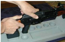
Insert the front end of the top cover into the rear sight block well. Lower the rear end of the cover and press it down, till it locks with the spring assembly. It is widely used to slam on the rear end of the top cover to quickly lock it in place. Before the magazine, pull the charging handle all the way to the back, allowing it to slam forward.
