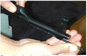
Removing cleaning rod. Here, it is clear of the retaining slot and may be moved forward and removed from the rifle. Locate the cleaning rod, with its front retained in a milled slot below the front sight. Grasp the rod just behind the front sight and bend it outward until it clears the retaining slot, and slide it forward until it clears the slot. You can then slide it on out of the rifle. This ends basic field-stripping, but you can proceed with a few more steps if you like.
