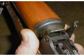
Remove the gas tube. On the right side of a rear sight block, locate the Gas Tube Release lever. Lift it some more to clear the rear sight and it will come right off. Locate the gas tube release lever, which is located on the right side of the rear sight, at the top forward corner. Rotate this lever clockwise by lifting upward on the rear of the lever. When the lever is vertical, you can lift the rear of the gas tube and remove it from the rifle.
