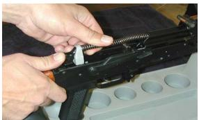
Insert the front end of the spring assembly into the round opening in the rear end of the carrier. Push the serrated button forward and align the railings, then release the button, allowing spring assembly to move backwards until set in place.
