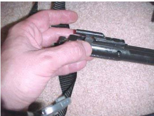
Next step you want to take out the pin that runs though the bolt, twist it a bit so it clears the gas tube on the bolt
