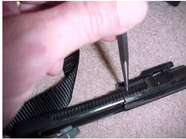
next we want to take the bolt apart. Take a small punch of the tip of a .223 round and push out the cotter pin in the rear of the bolt.
