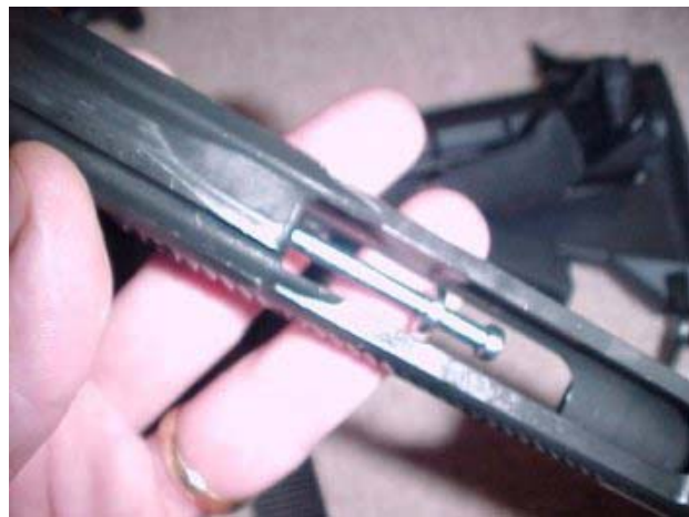
Tip the bolt on its back and the firing pin should come right out.
