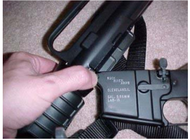
Also if you want you can totally separate the upper from the lower by taking out the other pin in the front. As for cleaning solvents, use break free CLP and some Hoppes #9. It helps to also have some Q-tips to clean where the bolt fits into the upper receiver and pipe cleaners for the gas tube as well.
