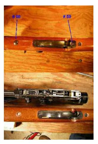
Pull out the assembly post, Mine came out with just my fingers. You might have to give yours a nudge on the bottom. It's plastic; so don't hit it with a punch.
