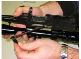
Insert bolt handle through the side of the receiver. With a screwdriver, push the bolt handle to the back until it snaps into the bolt assembly.
