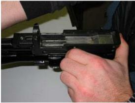
The bolt assembly is now at the back of the receiver...ready to be pulled out. Once the bolt stop pin has been removed, the bolt assembly can be removed by pulling the bolt handle to the back, this will cause the bolt assembly to follow. When it reaches the back of the receiver, the bolt assembly can be lifted out of the receiver.
