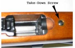
Before stripping the rifle make sure it is **UNLOADED!!! Removing the Stock** The first thing to do is to remove the stock. Most models will have a take-down screw near the magazine well and a barrel band.
