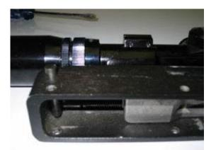
**Removing the Bolt Assembly** Once the trigger assembly has been removed from the receiver, the bolt assembly can be removed by first removing the bolt stop pin by pushing it through to the other side with a screwdriver of similar.
