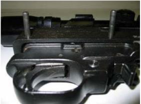
**Removing the Trigger Assembly** The trigger assembly can be removed by removing two cross pins which holds it to the receiver. This can be done by pushing the pins through the other side with a small screwdriver of other similar tool.
