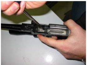
You will know that the two have snapped together as the bolt assembly will be able to go forward and follow the bolt handle with ease.
