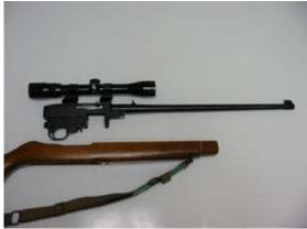
Once this is done, the stock should be able to slide off the rifle. The assembly slides straight out of the stock.)
