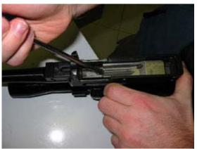
Once this is complete, you may reinstall the bolt stop pin back into its place.
