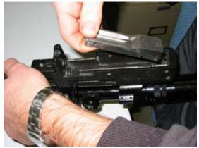
I have brought the bolt handle forward and now I'm lifting the bolt assembly out. When you lift the bolt assembly out, make sure you keep tension on the bolt handle and bring bolt handle back forward slowly (as I am doing in the above picture with my left hand. Failing to do so will cause the bolt handle to slam forward and may break.
