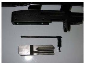
The bolt handle and bolt assembly. When reassembling the bolt assembly, redo the above steps backwards however you will need a screwdriver to assist you. You will need to insert the bolt handle first then place the bolt assembly into place. The two will need to lock together before the bolt can properly fit in its place.
