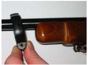
When removing the barrel band, be careful not to separate the ends too much as it may break. Once the take-down screw and barrel band have been removed, put the safety on in the middle position between the "on" (safe) and "off" (fire) position.
