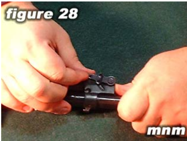
Rotate the gas cylinder latch to 10 o'clock position to keep the gas extension rod inside while you complete the next steps.
