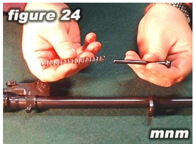
Separate the gas piston extension and spring and then set aside.
