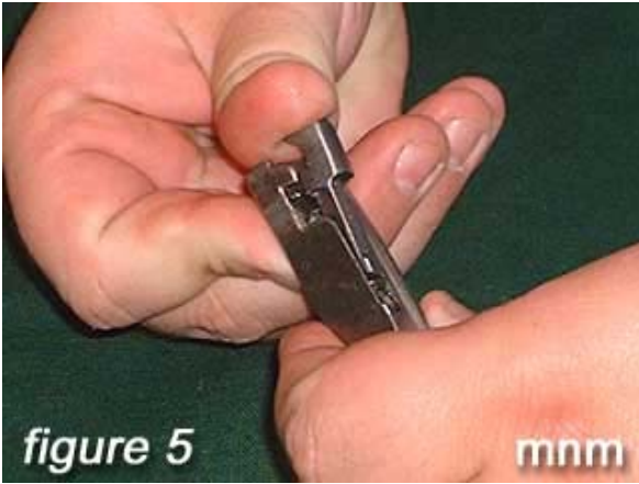
Snap the extractor back onto bolt body.
