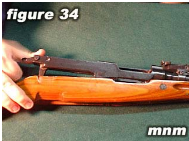
Place the receiver and barrel assembly back into stock (as shown in figures 21).
