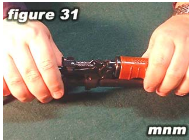
Make sure the end of the piston rod is flush with the end of the gas cylinder tube and then snap in down and into place.
