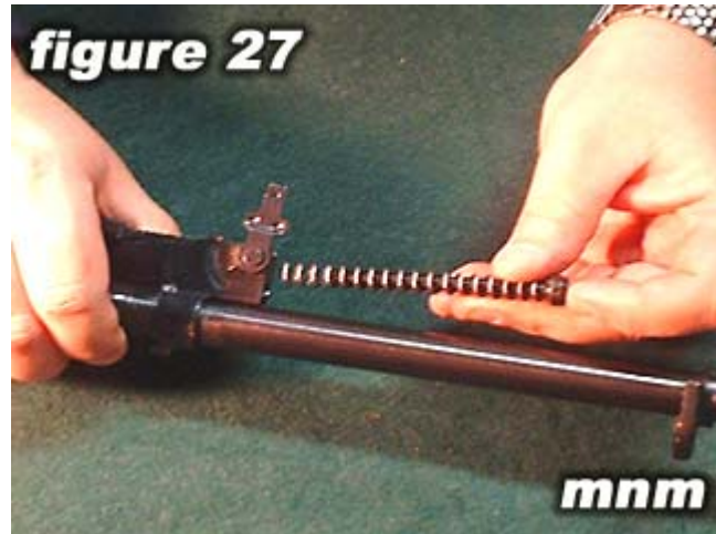
Insert the gas extension rod and spring back into the carbine.
