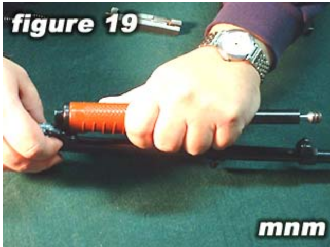
Pull the gas cylinder tube off of the gas cylinder. Take care not to allow the gas piston to fly out.
