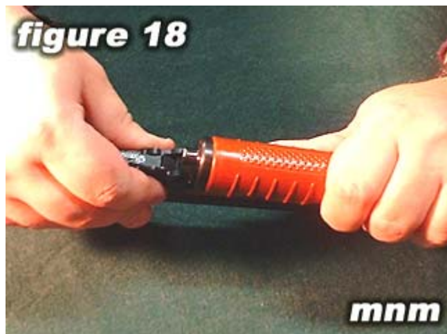
Pivot the gas cylinder tube at the front and lift the rear upwards.
