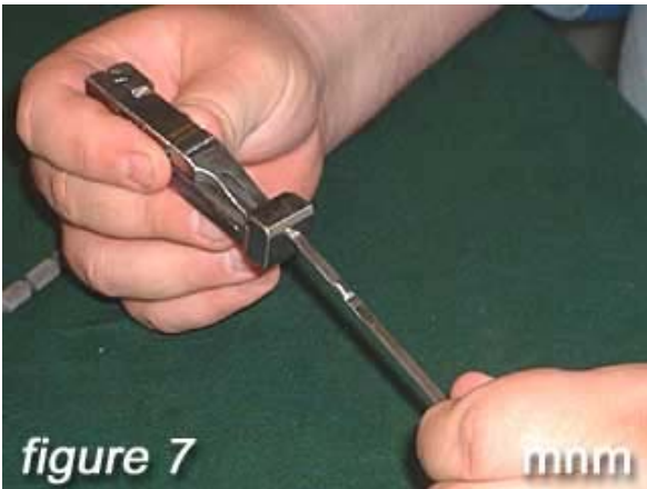
Reinsert the firing pin. Make certain that the firing pin is positioned inside the bolt so you can slide the firing pin retaining pin into the bolt body.
