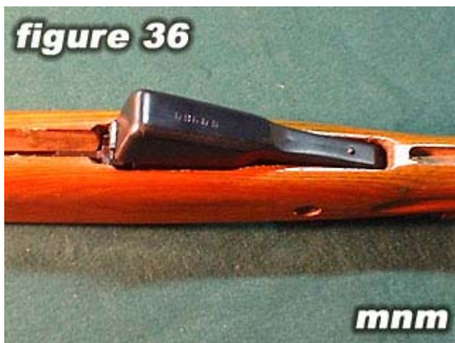
Correctly installed magazine.
