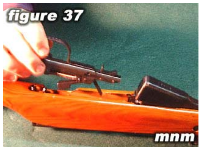
Take trigger assembly and line it up with slotted the guides inside of the receiver. See figure 38 below for help.
