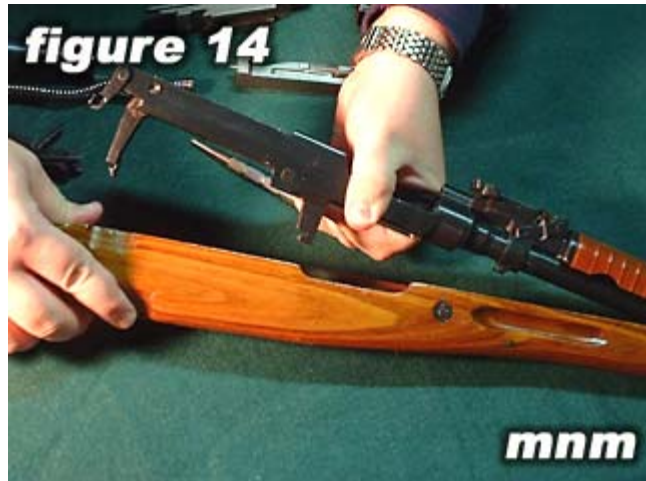
Pivot the barrel/receiver apart from the stock and set the stock aside.
