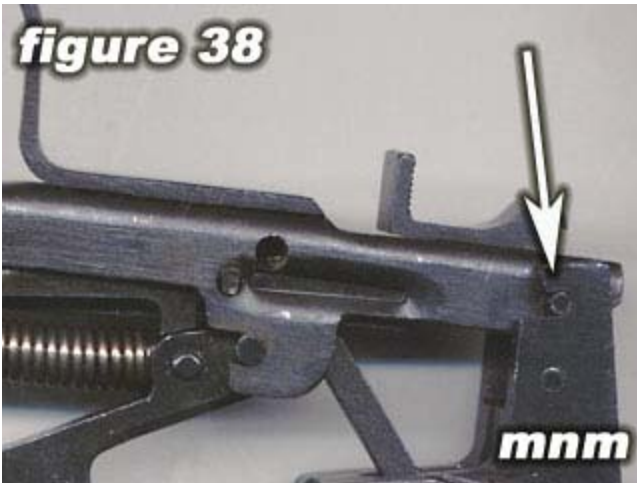
How the trigger assembly attaches to the receiver at below and at the rear of magazine.
