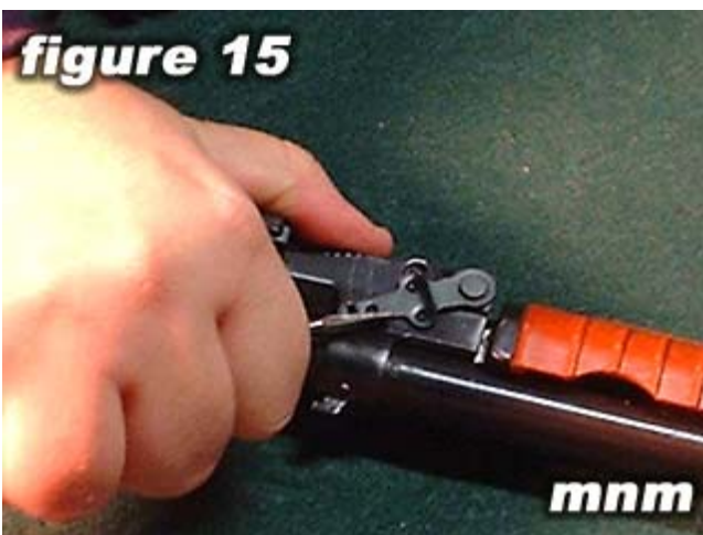
Rotate the gas cylinder tube latch clock-wise until it points to the 10 o'clock position if looking at the right side of carbine.
