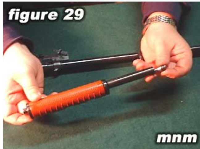
Place the gas piston into gas cylinder tube.
