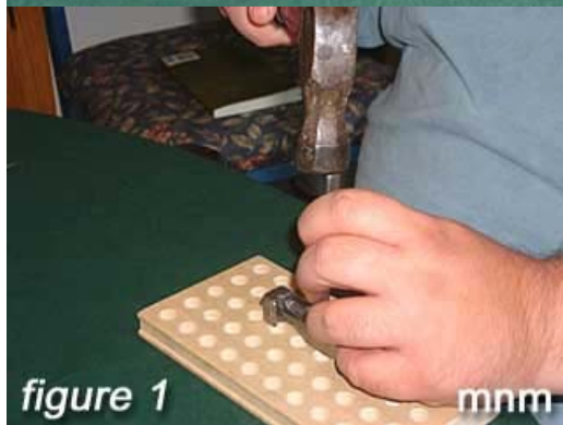
Using a punch, lightly tap out the firing pin retaining pin.
