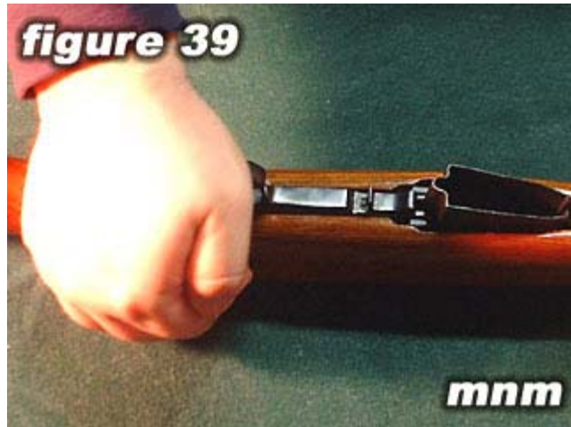
Pivot the trigger assembly back once engaged in guides inside receiver and then lock down the trigger assembly firmly with hand.
