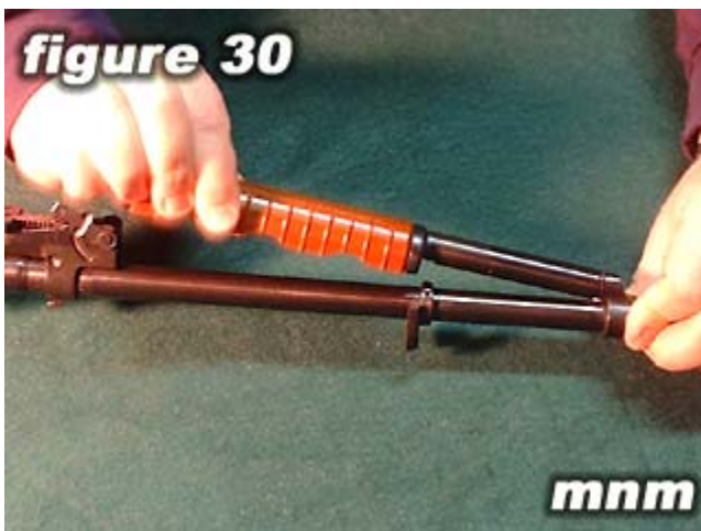
Attach the gas cylinder tube to gas cylinder.
