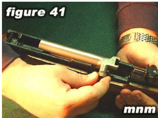
Install the bolt and bolt carrier into rear of receiver.
