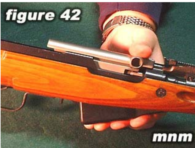
Slide the bolt and bolt carrier towards the front of receiver.
