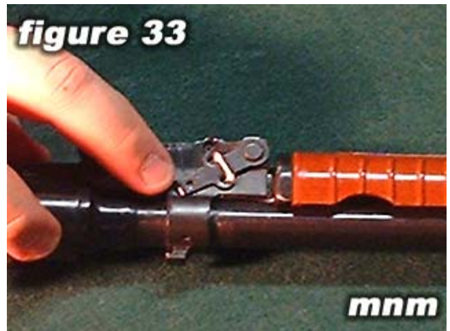
Lock the gas cylinder tube latch in place.
