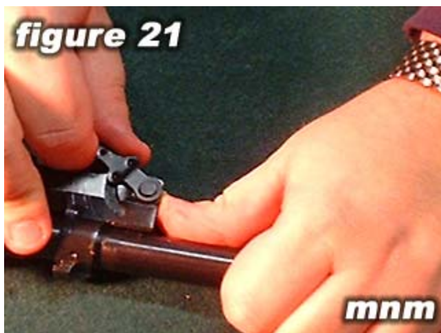
Make sure you hold your hand to prevent the gas piston extension from flying out of the carbine, as it is spring-loaded. Rotate the gas cylinder latch (as shown figure 22) to remove the gas piston extension.
