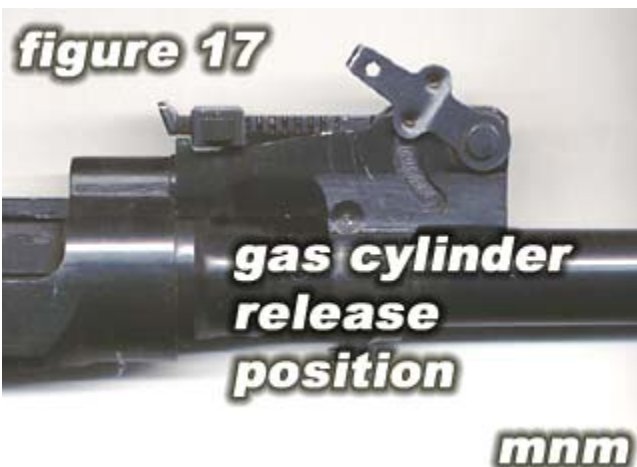
Figure 16 shows the gas cylinder tube latch in the 10 o'clock position that is required to remove the gas cylinder tube.
